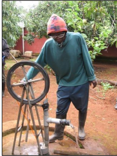
Figure 11: Owner of a Self-supply well in Njombe using his Rope Pump (Photo: Author)
