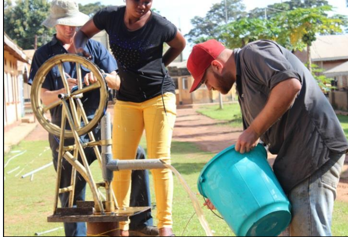
Figure 14: Testing trial of Rope Pump with female subject (Photo: Bosco Okot)
